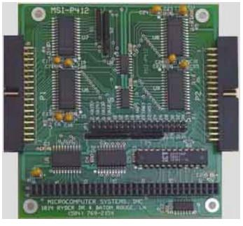
0-10V,  $\pm 5V$  and  $\pm 10V$  with a linearity of 1/2 LSB. In addition, the inputs are overvoltage tolerant to  $\pm 16.5V$  and a fault condition on any channel will not effect the conversion result on the selected channel.
