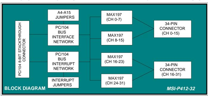
of each channel into a 12-bit digital signal. Low span and offset errors result in no adjustments being required for these functions. Typical total conversion times of 12 us gives a sample rate of 83 ksps for each group of eight channels yielding rates up to 332 ksps for 32 input channels.
